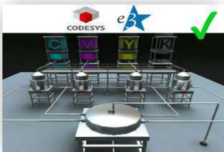
**Project:** the student is required to develop a SCADA system for the ink coloring process using the SCADA system Elipse E3. The reason is that the factory plans to build a control room for the operation of all its processes and machines.
