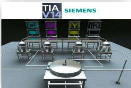
**Project:** the student is required to develop a SCADA system for the ink coloring process using the SCADA system WinCC.
